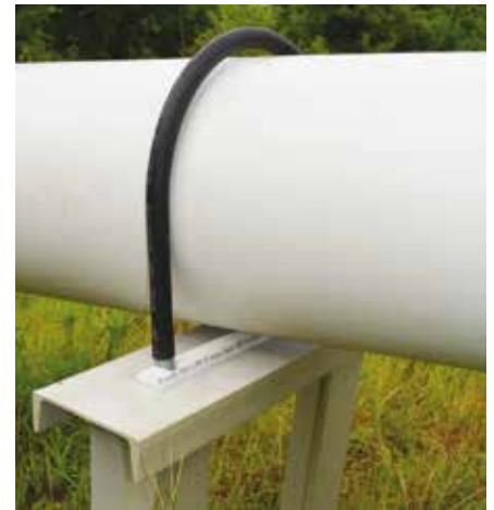
I-Rod® eliminates the crevice by minimizing the contact area and allowing any moisture to evaporate. It’s also much easier to inspect.
